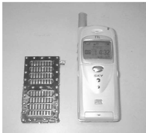
Fig. 2. Photograph of DMFC sub-module of four unit cells connected in series.
